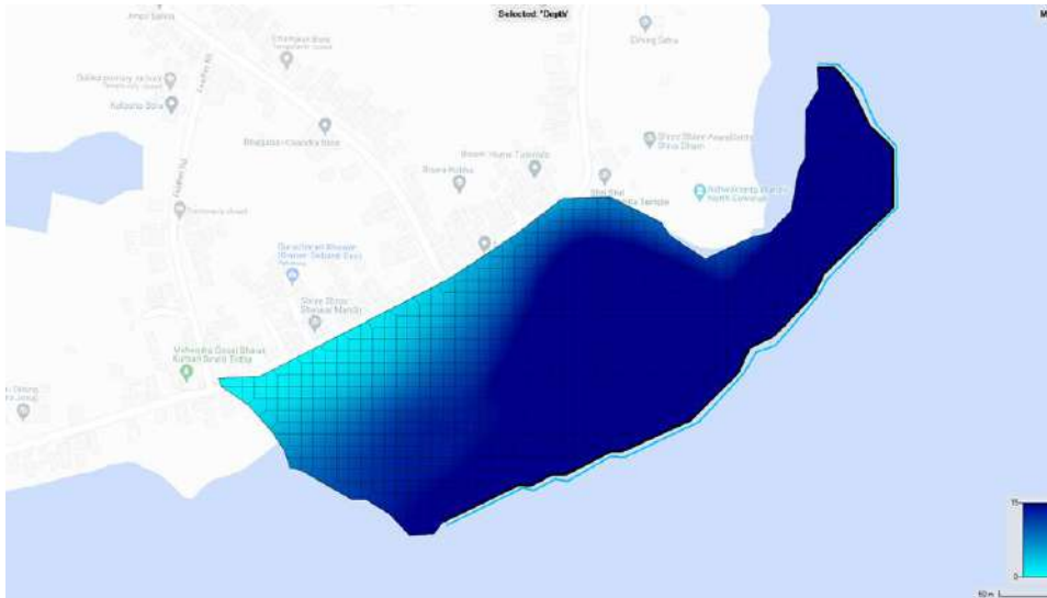
Figure 4-72: Simulated maximum depth (m) at North Guwahati
