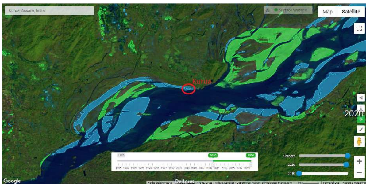
Figure 4-11 Aquamonitor images showing erosion and accretion changes from 2010 to 2020 ( https://aqua-monitor.appspot.com/ ) at Kurua (Blue colour polygon indicates: land has become water and green colour polygon indicates water has become land)
