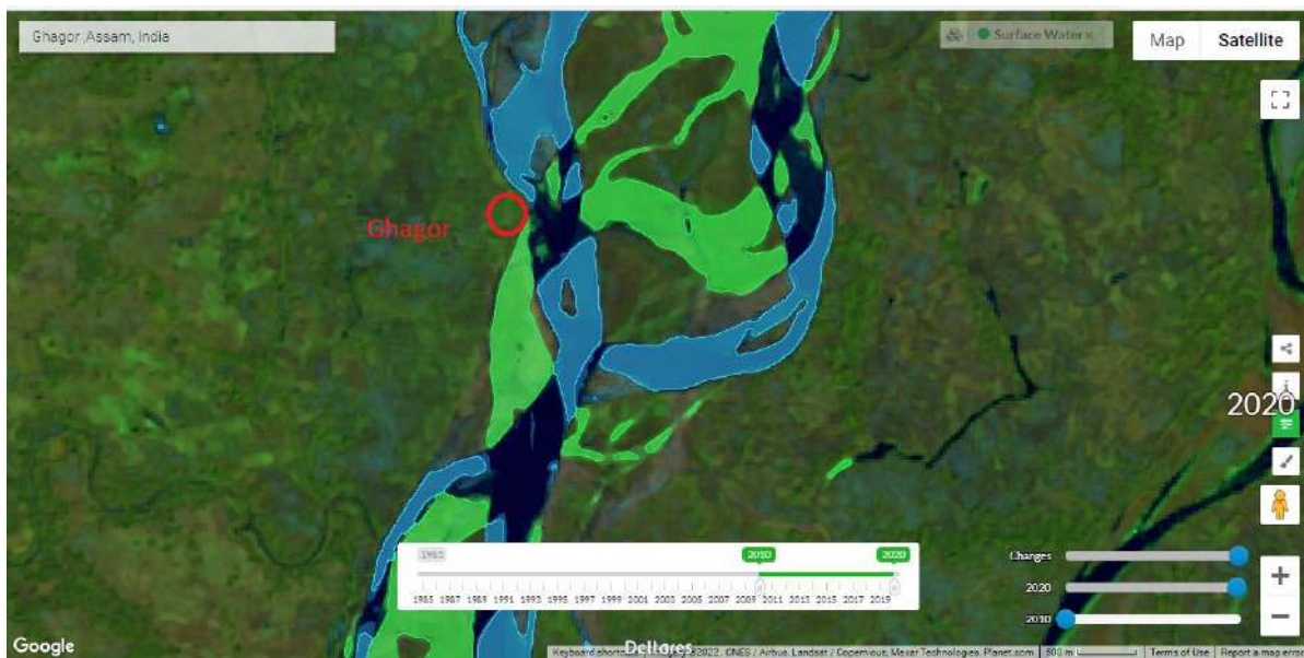
Figure 4-17 Aquamonitor images showing erosion and accretion changes from 2010 to 2020 ( https://aqua-monitor.appspot.com/ ) at Ghagor in the tributary Subansiri, Brahmaputra, (Blue colour polygon indicates land has become water and green colour polygon indicates water has become land)
