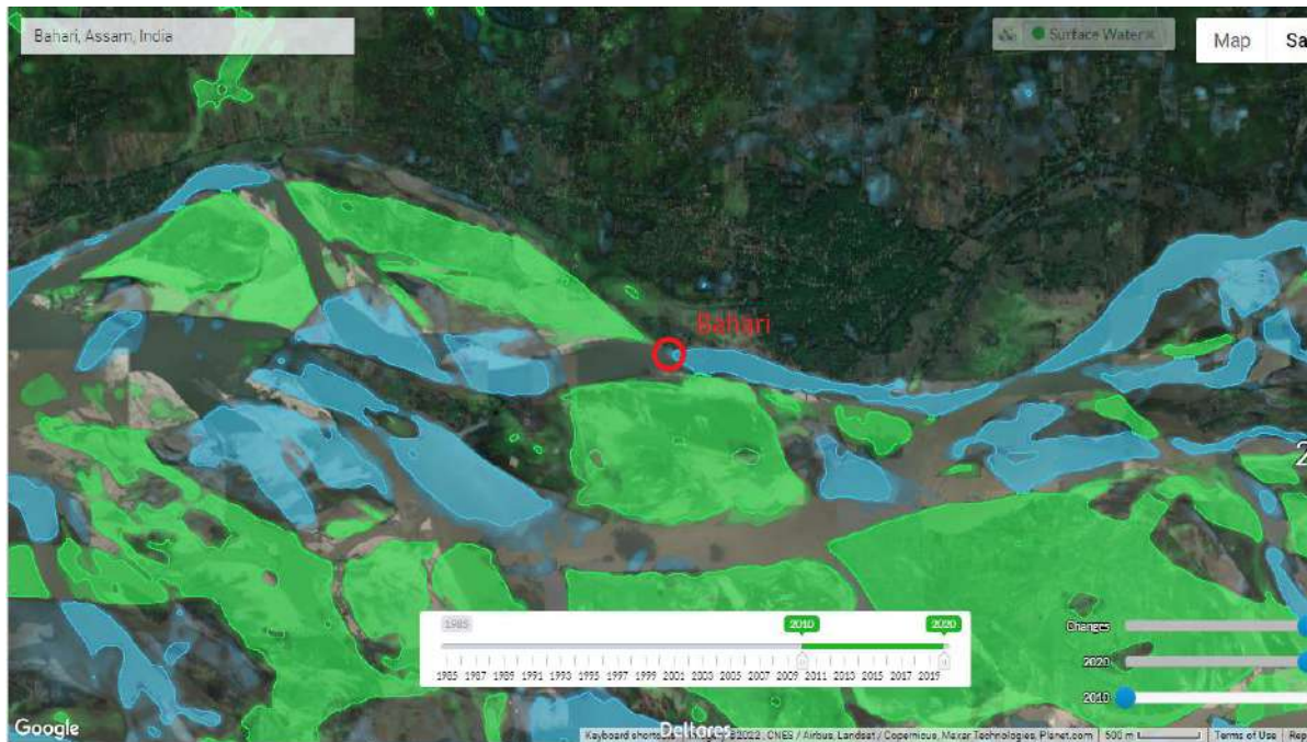
Figure 4-14 Aquamonitor images showing erosion and accretion changes from 2010 to 2020 ( https://aqua-monitor.appspot.com/ ) at Bahari (Blue colour polygon indicates: land has become water and green colour polygon indicates water has become land)
