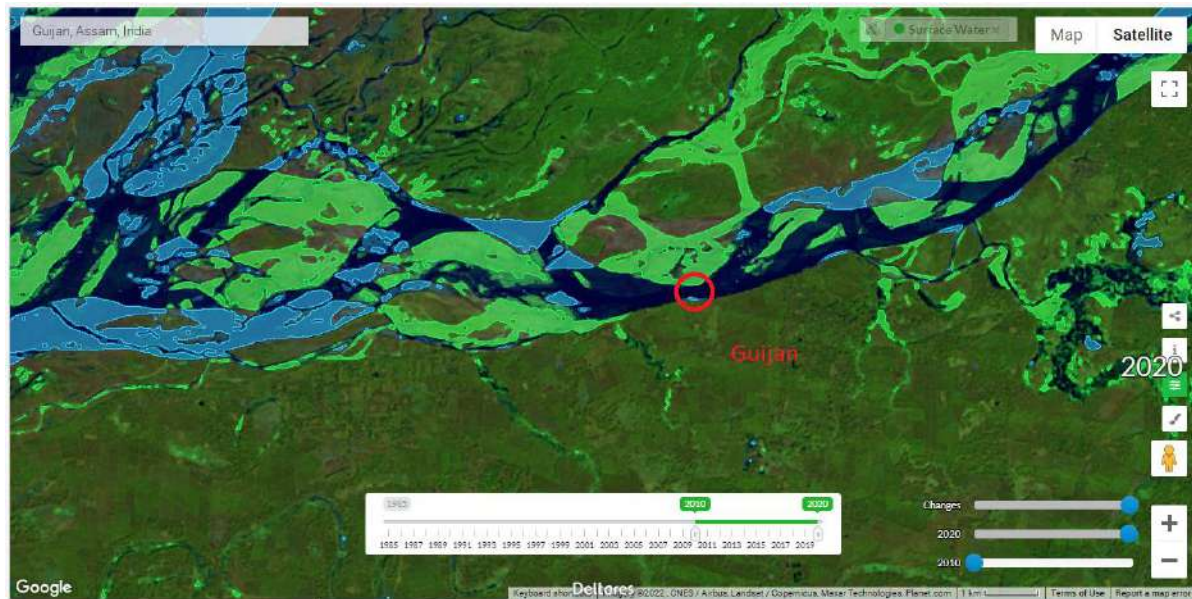
Figure 4-8 Aquamonitor images showing erosion and accretion changes from 2010 to 2020 ( https://aqua-monitor.appspot.com/ ) at Gujjan (Blue colour polygon indicates: land has become water and green colour polygon indicates water has become land)
