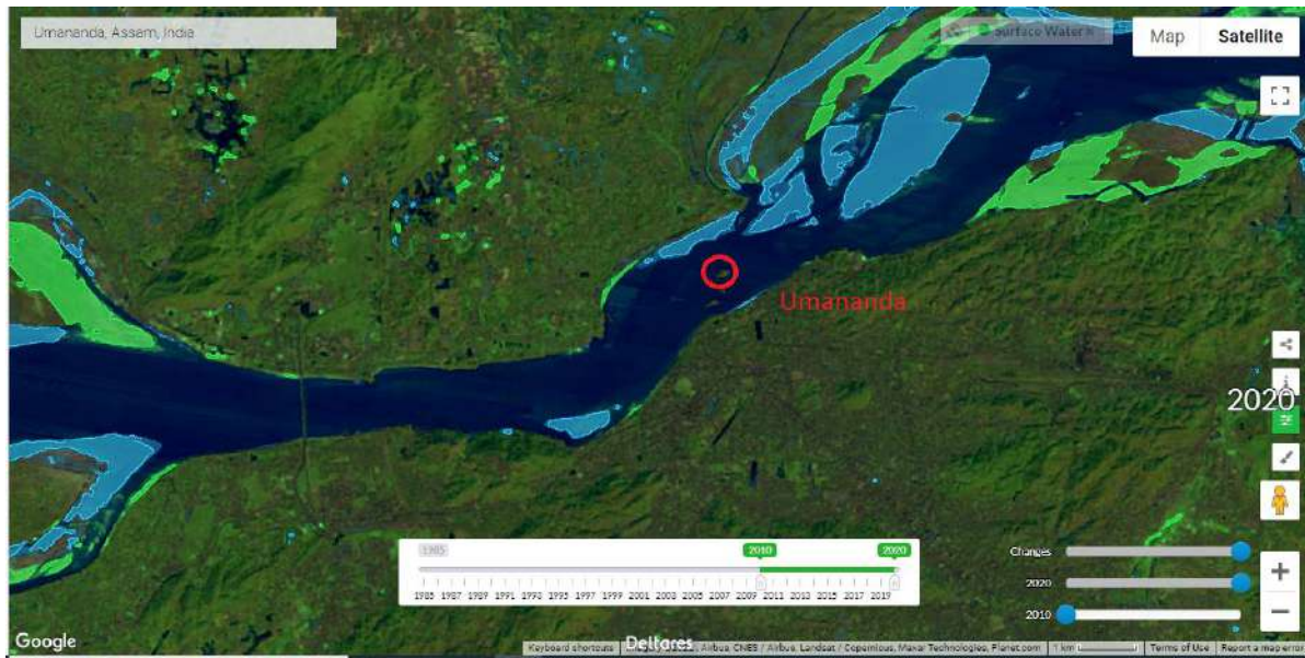
Figure 4-12 Aquamonitor images showing erosion and accretion changes from 2010 to 2020 ( https://aqua-monitor.appspot.com/ ) at Umananda (Blue colour polygon indicates: land has become water and green colour polygon indicates water has become land)
